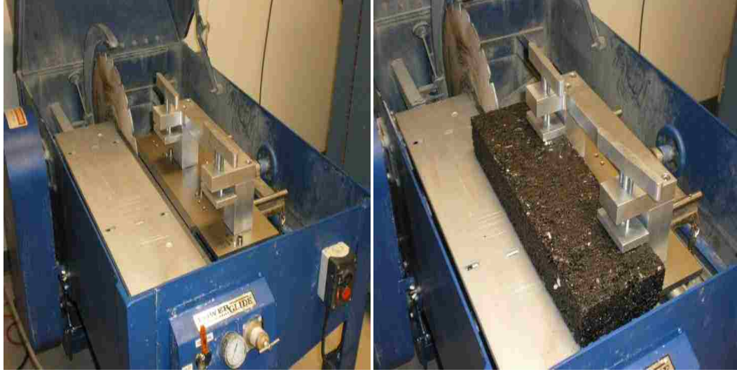
Figure 3.6 Stone Cutting Saw with Modified Clamp
