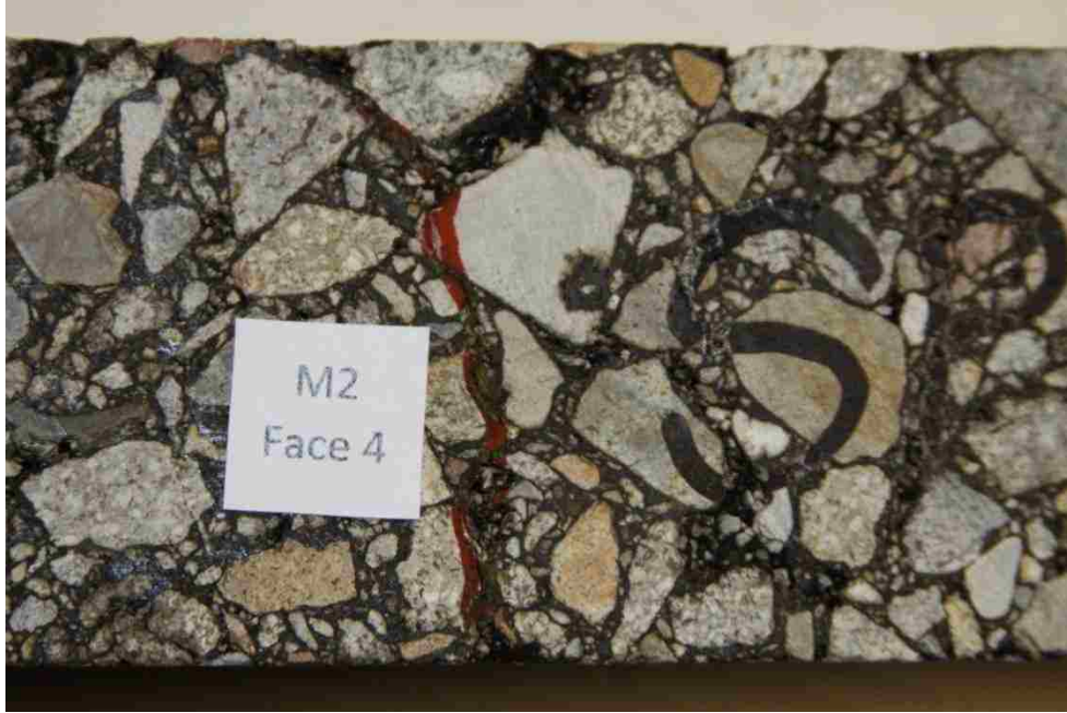
Figure 6.8 Fatigue Cracking in HMA Beam Sample SP-III-M2
