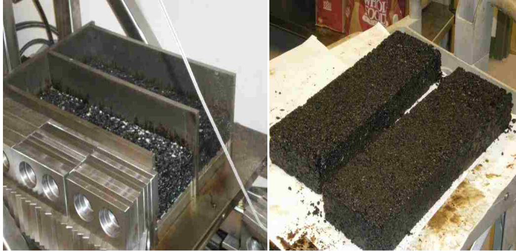
Figure 3.5 HMA Beam Samples Compacted by Linear Kneading Compactor
