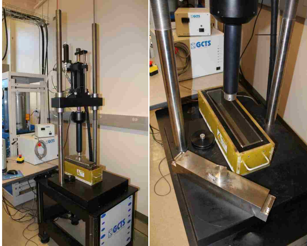
Figure 3.3 Loading Frame and Sample Mold for Beam Compaction
