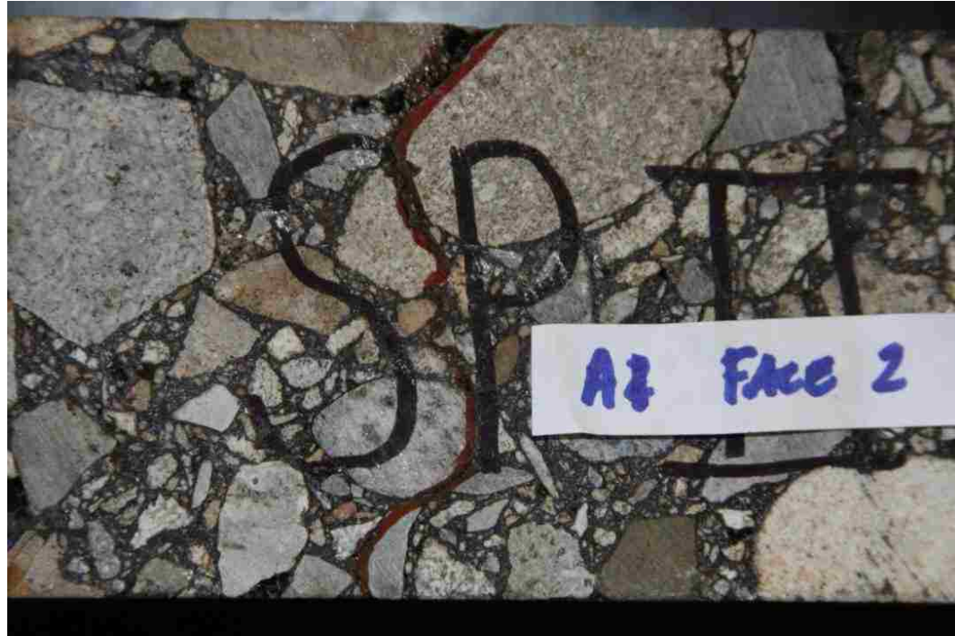
Figure 6.1 Fatigue Cracking in HMA Beam Sample SP-II-A1
