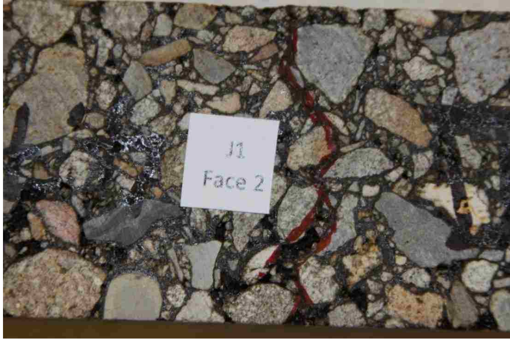
Figure 6.7 Fatigue Cracking in HMA Beam Sample SP-III-J1
